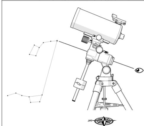
1.5 The approximate polar alignment is finished, when Polaris is visible in the centre of your field of view while looking through the empty polar tube. To move and centre Polaris there, it is necessary to finely adjust the mounts altitude and azimuth axis.
