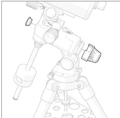
1.4 Remove the front and back polar scope covers. For an exact polar alignment, an optical polar scope can be installed here. For the approximate polar alignment, the naked view through the polar tube is enough.
