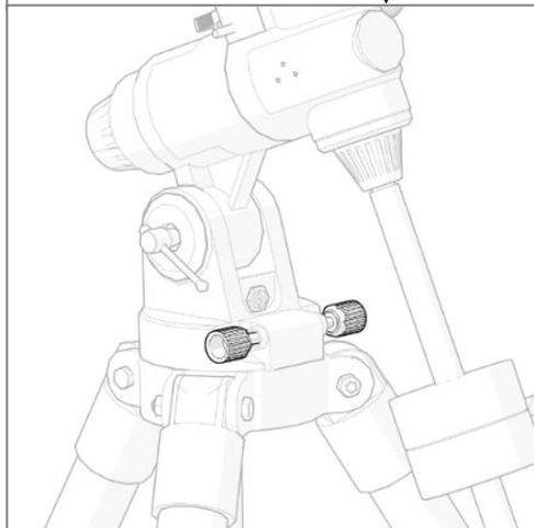
1.7 To move Polaris left and right in your field of view, you need to adjust the azimuth axis of the mount. Use the two azimuth adjustment screws for that. Screw them both in (without force) until you feel a resistance. The screws now clamp around a knob on top of the tripod. Now you must always operate both adjustment screws simultaneously: When screwing one adjustment further in, you must screw the other adjustment further out. This moves Polaris left or right in your field of view.
